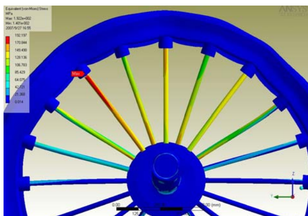
Figure 4: Equivalent stress (192.2 < 207 MPa)
